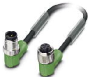
Sensor/actuator cable, 5-position, Variable cable type, Plug angled M12, A-coded, on Socket angled M12, A-coded, cable length: Free input (0.2 ... 40.0 m)
