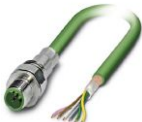
Bus system flush-type male connector, INTERBUS, 5-pos., M12, shielded, B-coded, front/screw mounting with M16 thread, can be positioned, with 0.5 m bus line
