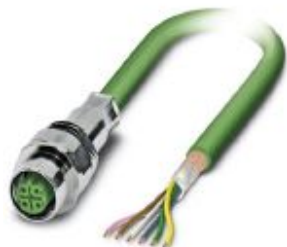
Bus system flush-type female connector, INTERBUS, 5-pos., M12, shielded, B-coded, front/screw mounting with M16 thread, can be positioned, with 0.5 m bus line
