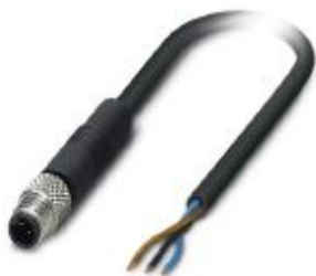
Sensor/actuator cable, 3-position, PUR, black RAL 9005, Plug straight M5, coding: A, on free cable end, cable length: 3 m
