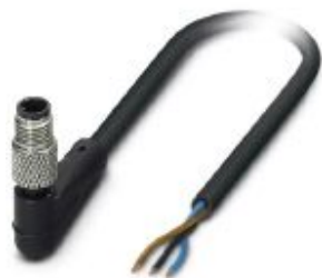
Sensor/actuator cable, 3-position, PUR, black RAL 9005, Plug angled M5, coding: A, on free cable end, cable length: 1.5 m
