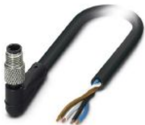
Sensor/actuator cable, 4-position, PUR, black RAL 9005, Plug angled M5, coding: A, on free cable end, cable length: 10 m
