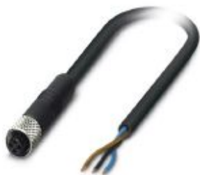
Sensor/actuator cable, 3-position, PUR, black RAL 9005, free cable end, on Socket straight M5, coding: A, cable length: 5 m
