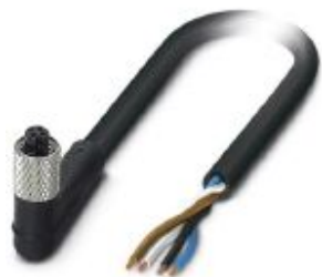
Sensor/actuator cable, 4-position, PUR, black RAL 9005, free cable end, on Socket angled M5, coding: A, cable length: 1.5 m
