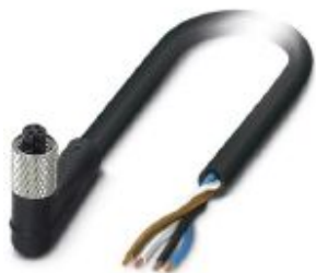
Sensor/actuator cable, 4-position, PUR, black RAL 9005, free cable end, on Socket angled M5, coding: A, cable length: 3 m
