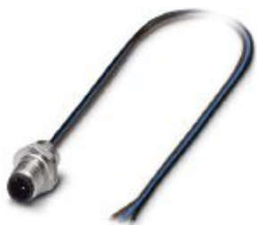
Sensor/actuator flush-type plug, 3-pos., M5, prewall/screw mounting, with M5 thread, with 0.5 m TPE litz wire, 3 x 0.14 mm 2
