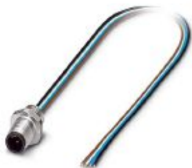
Flush-type connector, 4-position, Plug, straight, M5, Front mounting, M5 x 0.5, Individual wires, cable length: 0.5 m, 0.14 mm 2 , TPE litz wire
