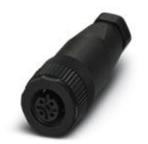
Bus system connector, 5-position, Socket straight M12, B-coded, Screw connection, knurl material: Plastic, cable gland Pg9, external cable diameter 6 mm ... 8 mm
