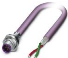
Bus system flush-type plug, PROFIBUS, 2-pos., M12, shielded, B-coded, rear/screw mounting with M16 thread, with 0.5 m bus cable, 2 x 0.25 mm 2
