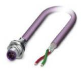
Bus system flush-type plug, PROFIBUS, 2-pos., M12, shielded, B-coded, rear/screw mounting with M16 thread, with 1 m bus cable,  $2 \times 0.25 \text{ mm}^2$
