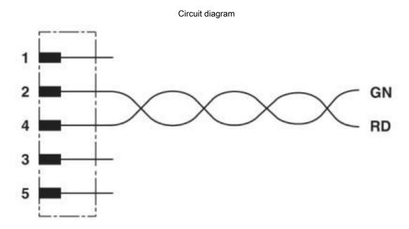
Contact assignment of the M12 plug
