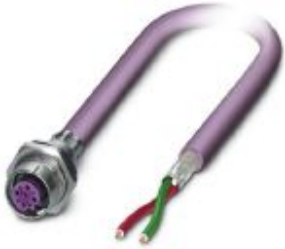
Bus system flush-type socket, PROFIBUS, 2-pos., M12, shielded, B-coded, rear/screw mounting with M16 thread, with 2 m bus cable, 2 x 0.25 mm 2
