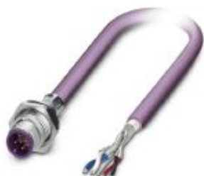
Bus system flush-type plug, DeviceNet/CANopen, 5-pos., M12, shielded, A-coded, rear/screw mounting with M16 thread, with 1 m bus cable, 2 x 0.2 mm 2 , 2 x 0.32 mm 2
