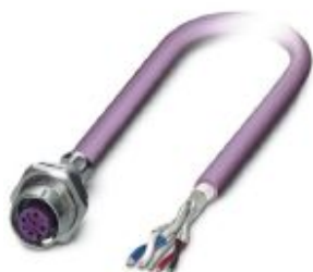
Bus system flush-type socket, DeviceNet/CANopen, 5-pos., M12, shielded, A-coded, rear/screw mounting with M16 thread, with 2 m bus cable, 2 x 0.2 mm 2 , 2 x 0.32 mm 2
