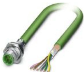
Bus system flush-type male connector, INTERBUS, 5-pos., M12, shielded, B-coded, rear/screw mounting with M16 thread, with 2 m bus line
