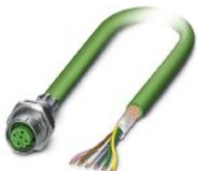
Bus system flush-type female connector, INTERBUS, 5-pos., M12, shielded, B-coded, rear/screw mounting with M16 thread, with 1 m bus line
