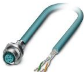
Bus system flush-type socket, Ethernet, 4-pos., M12, shielded, D-coded, rear/screw mounting with M16 thread, with 0.5 m bus cable, 2 x 2 x 0.14 mm 2
