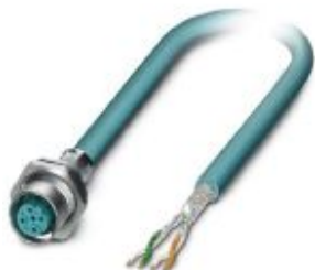
Bus system flush-type socket, Ethernet, 4-pos., M12, shielded, D-coded, rear/screw mounting with M16 thread, with 1 m bus cable, 2 x 2 x 0.14 mm 2
