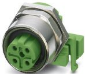
Bus system flush-type socket, Ethernet, 4-pos., M12, shielded, D-coded, rear/screw mounting, with angled solder connection
