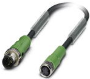
Sensor/actuator cable, 3-position, PUR halogen-free, black-gray RAL 7021, Plug straight M12 SPEEDCON, A-coded, on Socket straight M8, cable length: 1 m
