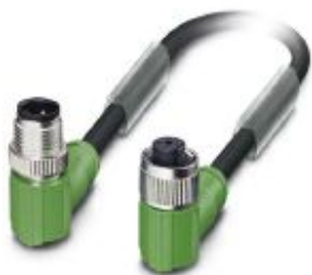
Sensor/actuator cable, 4-position, Variable cable type, shielded, Plug angled M12, coding: A, on Socket angled M12, coding: A, cable length: Free input (0.2 ... 40.0 m)
