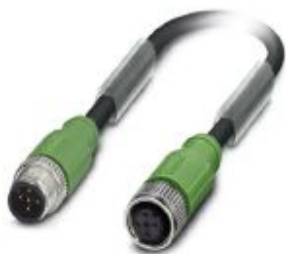
Sensor/actuator cable, 5-position, Variable cable type, shielded, Plug straight M12, coding: A, on Socket straight M12, coding: A, cable length: Free input (0.2 ... 40.0 m)
