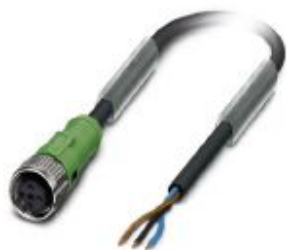
Sensor/actuator cable, 3-position, PUR halogen-free, black-gray RAL 7021, free cable end, on Socket straight M12 SPEEDCON, coding: A, cable length: 1.5 m
