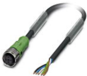
Sensor/actuator cable, 5-position, PUR halogen-free, black-gray RAL 7021, free cable end, on Socket straight M12 SPEEDCON, A-coded, cable length: 1.5 m
