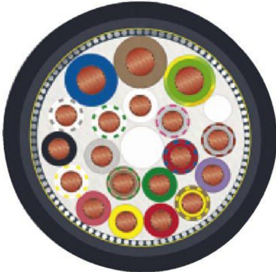
Cable cross section
