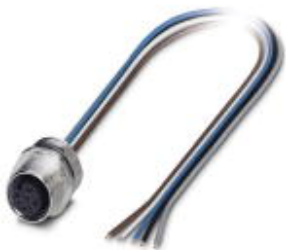
Sensor/Actuator flush-type socket, 5-pos., M12, A-coded, front/screw mounting with M16 thread, with 2.5 m TPE litz wire, 5 x 0.34 mm 2
