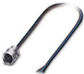
Panel feed-through, 3-position, Socket, straight, M8, Front mounting, M8 x 0.5, Individual wires, cable length: 1 m, 0.25 mm 2 , PVC litz wire
