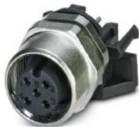
Sensor/actuator flush-type connector, socket, 5-pos., M12 SPEEDCON, A-coded, rear/screw mounting with M12 thread, with polarity protection, with straight solder connection
