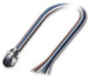
Flush-type connector, 6-position, Plug, straight, M8, Front mounting, M8 x 0.5, Individual wires, cable length: 0.5 m, 0.14 mm 2 , PVC litz wire
