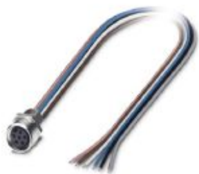
Flush-type connector, 6-position, Socket, straight, M8, Front mounting, M8 x 0.5, Individual wires, cable length: 0.5 m, 0.14 mm 2 , PVC litz wire
