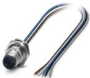
Sensor/actuator flush-type plug, 5-pos., M12 SPEEDCON, A-coded, rear/screw mounting with Pg9 thread, with 0.5 m TPE litz wire, 5 x 0.34 mm 2
