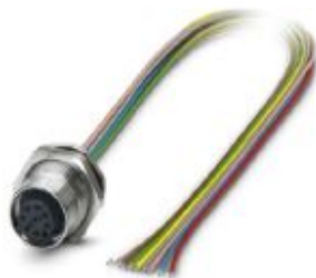
Sensor/actuator flush-type socket, 8-pos., M12 SPEEDCON, rear/screw mounting with Pg9 thread, with 0.5 m TPE litz wire, 8 x 0.25 mm 2
