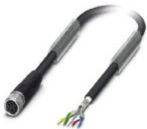
Bus system cable, INTERBUS, 4-position, PUR halogen-free, black RAL 9005, shielded, free cable end, on Socket straight M8, cable length: 20 m
