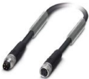
Bus system cable, INTERBUS, 4-position, PUR halogen-free, black RAL 9005, shielded, Plug straight M8, on Socket straight M8, cable length: 0.13 m
