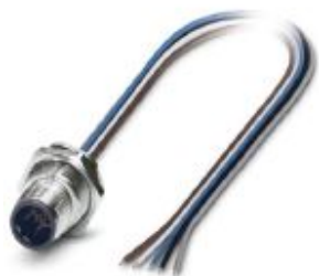
Sensor/actuator flush-type connector, 5-pos., M12 SPEEDCON, B-coded, rear/screw mounting with Pg9 thread, with 0.5 m TPE litz wire, 5 x 0.34 mm 2
