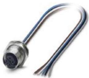
Sensor/actuator flush-type socket, 5-pos., M12 SPEEDCON, B-coded, rear/screw mounting with Pg9 thread, with 0.5 m TPE litz wire, 5 x 0.34 mm 2
