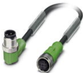
Sensor/actuator cable, 4-position, PUR, black-gray RAL 7021, Plug angled M12, A-coded, on Socket straight M12, A-coded, cable length: 5 m
