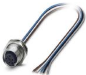
Sensor/actuator flush-type socket, 5-pos., M12, A-coded, rear/screw mounting with Pg9 thread, with 0.5 m TPE litz wire, 5 x 0.5 mm 2
