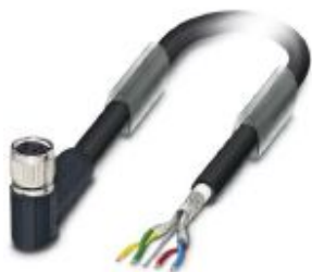
Bus system cable, INTERBUS, 4-position, PUR halogen-free, black RAL 9005, shielded, free cable end, on Socket angled M8, cable length: 5 m
