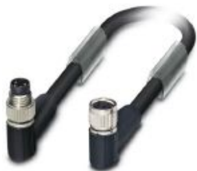
Bus system cable, INTERBUS, 4-position, PUR halogen-free, black RAL 9005, shielded, Plug angled M8, on Socket angled M8, cable length: 0.13 m
