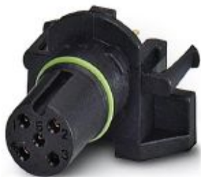
Sensor/actuator flush-type socket, 5-pos., A-coded, with straight solder connection, only contact insert
