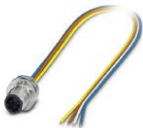
Bus system flat-type plug, PROFINET, 4-position, Plug, straight, M12-SPEEDCON, D-coded, Front mounting, M16 x 1.5, Individual wires, cable length: 0.5 m, 0.34 mm 2 , TPE litz wire
