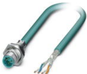
Bus system flush-type plug, Ethernet, 4-pos., M12 SPEEDCON, shielded, D-coded, rear/screw mounting with M16 thread, with 0.5 m bus cable, 2 x 2 x 0.2 mm 2
