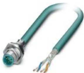
Bus system flush-type plug, Ethernet, 4-pos., M12 SPEEDCON, shielded, D-coded, rear/screw mounting with M16 thread, with 1 m bus cable, 2 x 2 x 0.2 mm 2
