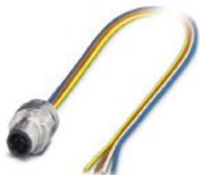
Bus system flat-type plug, 4-position, Plug, straight, M12-SPEEDCON, D-coded, Front mounting, can be positioned, M16 x 1.5, Individual wires, cable length: 0.5 m, 0.34 mm 2 , TPE litz wire
