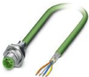
Bus system flush-type plug, PROFINET, 4-pos., M12, shielded, D-coded, rear/screw mounting with M16 thread, with 1 m bus cable, 2 x 2 x 0.34 mm 2
