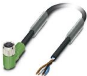
Sensor/actuator cable, 4-position, PUR halogen-free, black-gray RAL 7021, free cable end, on Socket angled M8, cable length: 15 m
